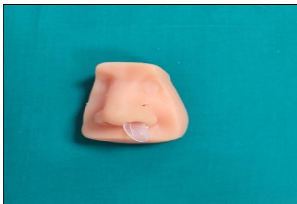
Figure 4: Insertion of Bi-Valve Splints into the Nasal Simulation Model for Evaluation
